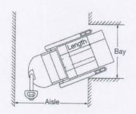
Aisle dimensions listed above assume the minimum bay width to be straddle OD plus 5" (2.5" on either side of straddle leg). Straddle OD is the load width plus 8". Truck performance may vary due to application requirements' and changes in model design.
